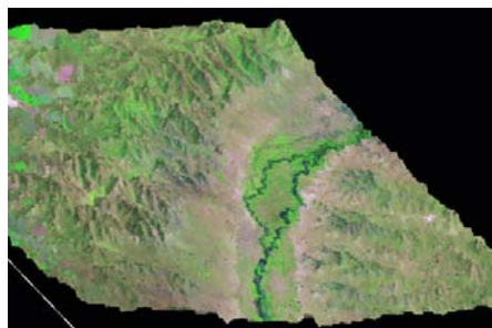
Three-dimensional representation of a DEM as processed from SPOT and LANDSAT data. Mongolia.
